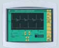
Example of acquisition of a secondary wave form signal (ignition)
